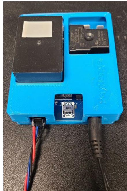
4-wire Harness connection to Mechanical Timer Module
