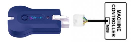
**5.** Restore power to machine -- after machine controller is fully booted, BluCheck status LED should turn solid blue.
